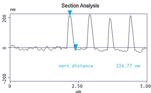
**Figure 3** (online colour at: [www.pss-a.com](http://www.pss-a.com)) AFM section analysis of a  $200\ \text{nm}$  diameter stamp, the vertical distance between the two arrows and hence height of the features is shown to be  $\sim 225\ \text{nm}$ .
