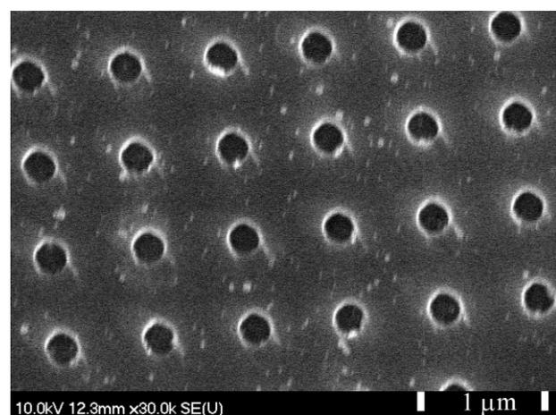
**Figure 4** SEM image of cpTi surface following imprinting using a UNCD stamp with  $200\ \text{nm}$  diameter features and a load of  $200\ \text{kg}$ .
