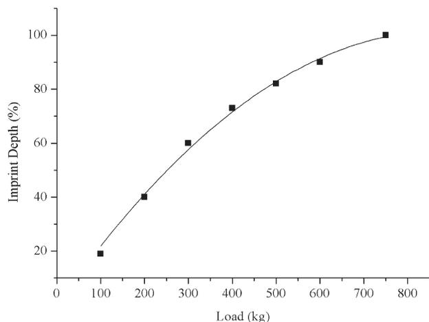
**Figure 6** Graph of imprint depth against applied pressing load for a UNCD stamp of side 250 μm containing 200 nm diameter circular pillars with 560 nm pitch into polished, planar cpTi. The depth is measured as a percentage with reference to feature height (100% = 225 nm).
