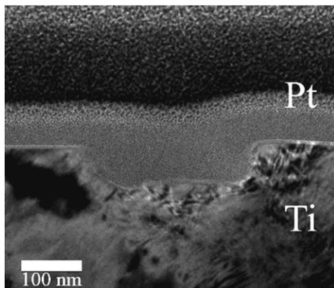
**Figure 5** TEM cross-section image of a single feature site on cpTi after imprinting with a UNCD stamp of feature diameter 200 nm at a load of 100 kg. The imprint is 50 nm deep and the Ti is covered with Pt for protection. The Pt was deposited with two separate induction beams which has produced two visually distinct layers.
