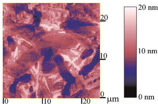
**Figure 1** (online colour at: [www.pss-a.com](http://www.pss-a.com)) AFM 25 μm square scan of cpTi surface after polishing. Image  $R_a = 2.352$  nm.
