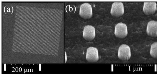
**Figure 2** (a) SEM over-view image of a pillar matrix stamp etched into UNCD with side  $250\ \mu\text{m}$  consisting of  $200\ \text{nm}$  diameter circular pillars at  $560\ \text{nm}$  pitch. (b) Close-up SEM image of  $200\ \text{nm}$  pillars at  $45$  degree tilt.
